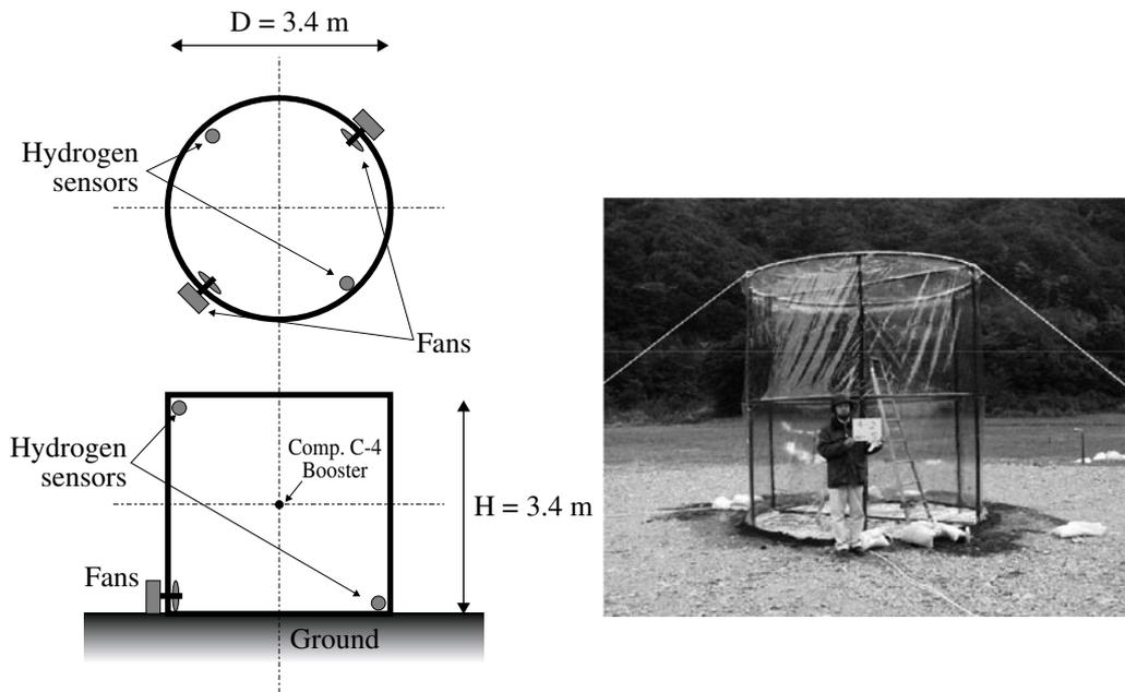
Fig. 1 Experimental setup for explosion test.
