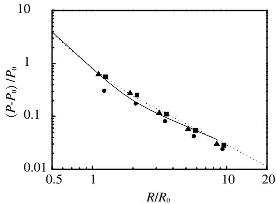
Fig. 4 Scaled peak overpressure with different hydrogen concentrations.
