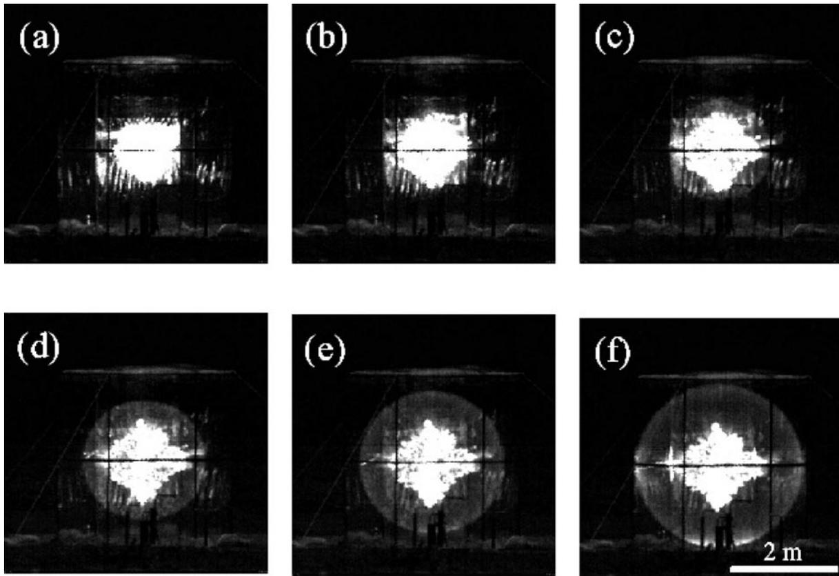
Fig. 2 Typical results of high-speed photography obtained during the explosion test with 52.9 vol.% hydrogen-air mixture, (a): 228  $\mu$ s, (b): 328  $\mu$ s, (c): 428  $\mu$ s, (d): 528  $\mu$ s, (e): 628  $\mu$ s, (f): 728  $\mu$ s after ignition of Composition C-4.
