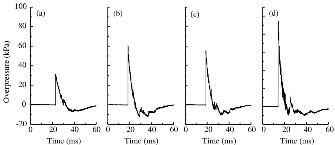
Fig. 3 Pressure wave histories with different hydrogen concentrations measured at same distance (10.6 m), (a): 21.0 vol.%, (b): 28.7 vol.%, (c): 52.9 vol.%, (d) shows typical blast wave profile generated by explosion of 20 kg TNT explosive.
