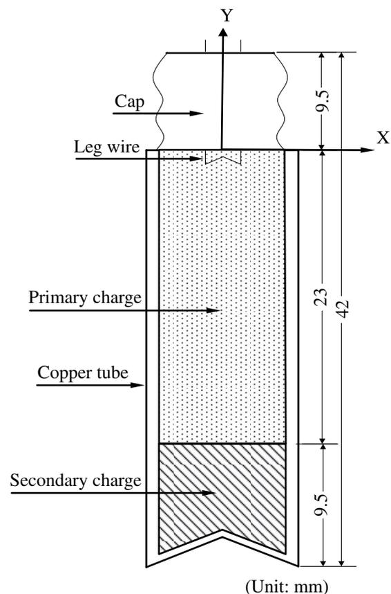
Fig. 1 Configuration of precise detonator.
