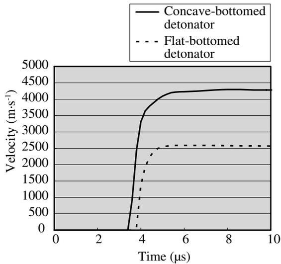
Fig. 6 The tip-velocity vs time.
