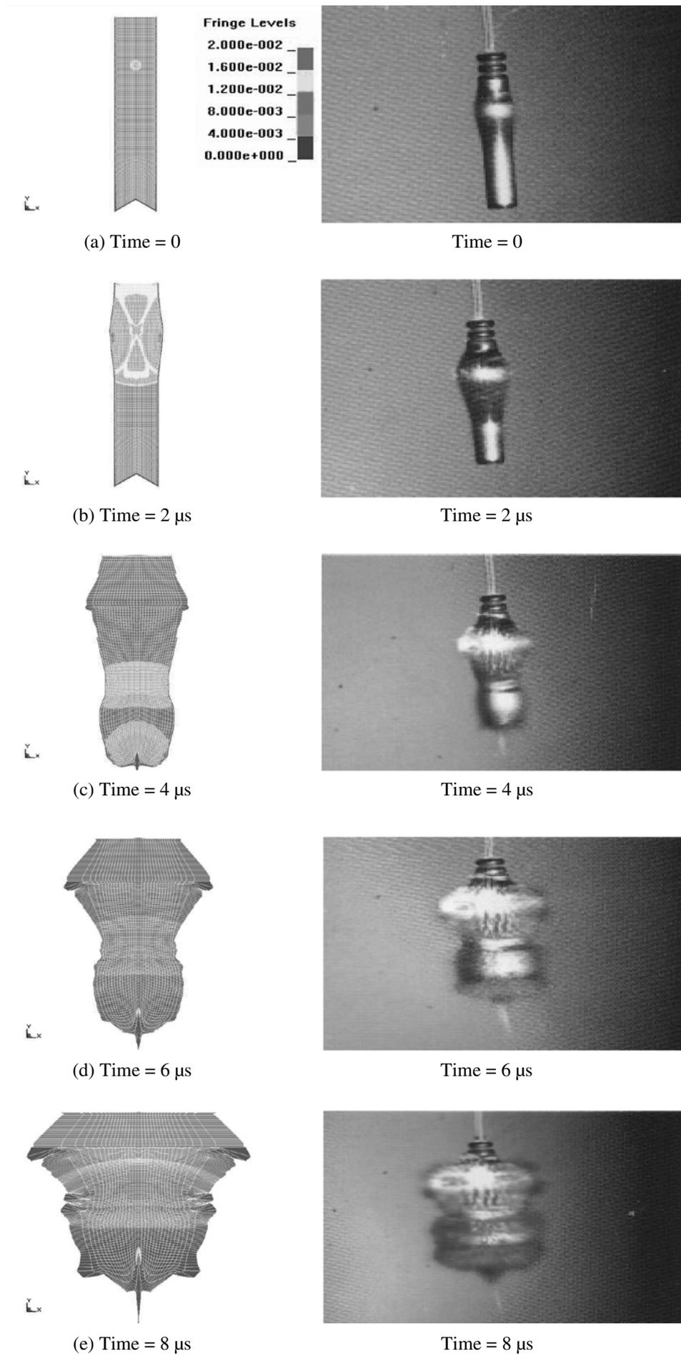
Fig. 3 The results of simulation and experiment of concave-bottomed detonator (contour of pressure).
