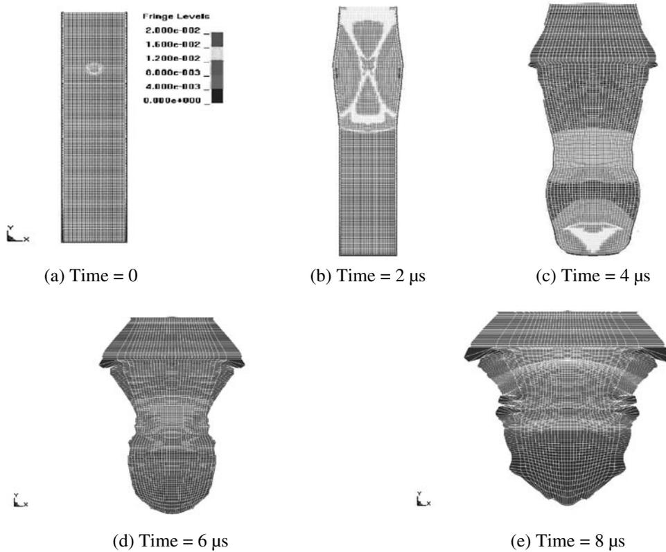
Fig. 5 The simulation results of flat-bottomed detonator (contour of pressure).
