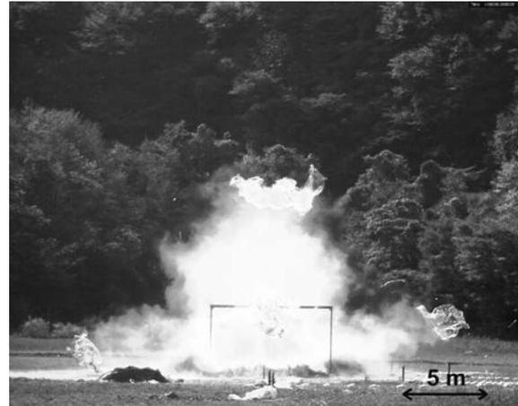
Fig. 2 Typical photograph of explosion phenomenon of hydrogen-air mixture with volumes of  $200 \text{ m}^3$ , taken at 400 ms after an electric spark ignition.
