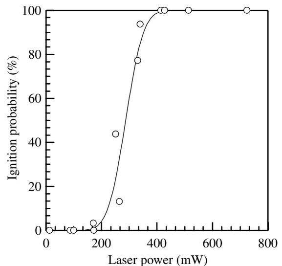
Fig. 6 Laser ignition probability of B/KNO<sub>3</sub> in vacuum, dependence on laser power.
