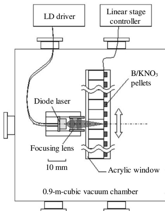
Fig. 1 Schematic diagram of the experimental setups.
