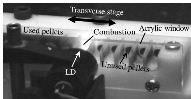
Fig. 3 Picture of the experimental setups.
