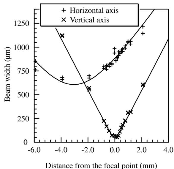
Fig. 2 Profiles of beam widths along the laser beam axis measured by a beam profiler.
