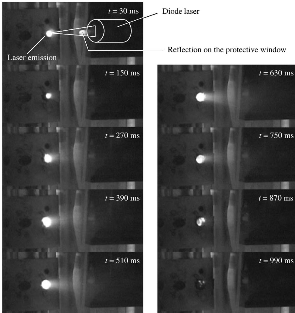
Fig. 5 Succeeding pictures of laser-ignited combustion of B/KNO<sub>3</sub> in vacuum.
