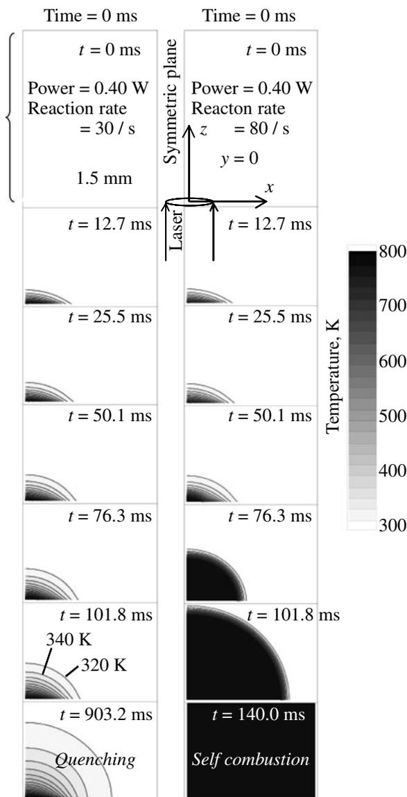
Fig. 7 Calculated temperature profiles on  $y = 0$  plane; comparison of the quenching (reaction rate of 30  $\text{s}^{-1}$ ) and self-sustained combustion (reaction rate of 80  $\text{s}^{-1}$ ).
