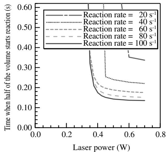
Fig. 9 Calculated ignition time when 55 % of volume starts the reaction ( $w_y = 50 \mu\text{m}$ ).
