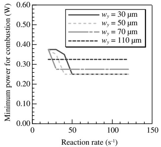
Fig. 8 Calculated minimum power necessary for the self combustion.
