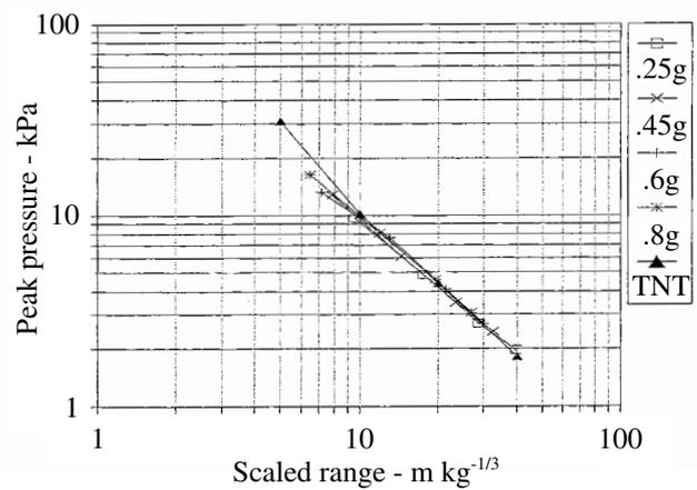
Fig. 2 Peak pressure versus scaled range in free air for detonators with various PETN base charges and for cast TNT.
