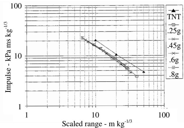
Fig. 4 Scaled impulse versus scaled range in free air for detonators with various PETN base charges and for cast TNT.
