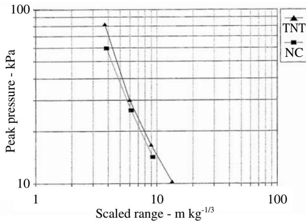
Fig. 1 Peak pressure versus scaled range for cellulose nitrate and cast TNT.
