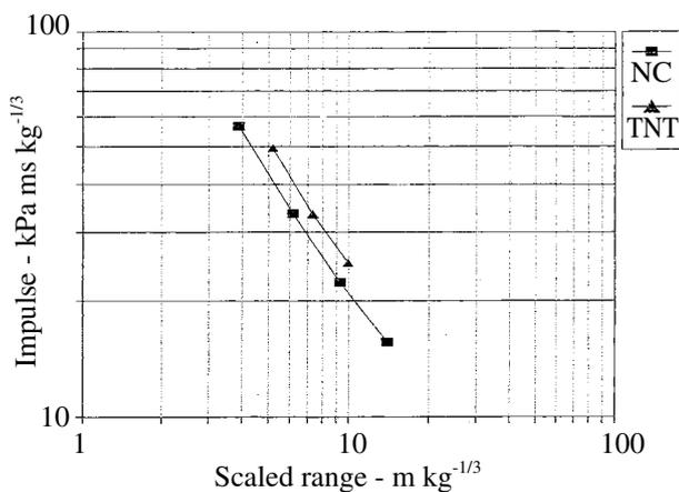
Fig. 3 Scaled impulse versus scaled range for cellulose nitrate and cast TNT.
