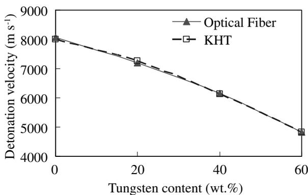
Fig. 1 Detonation velocity vs. tungsten content (wt.%).
