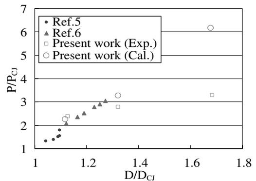
Fig. 11 Relation between pressure and velocity of the overdriven detonation for various explosives.
