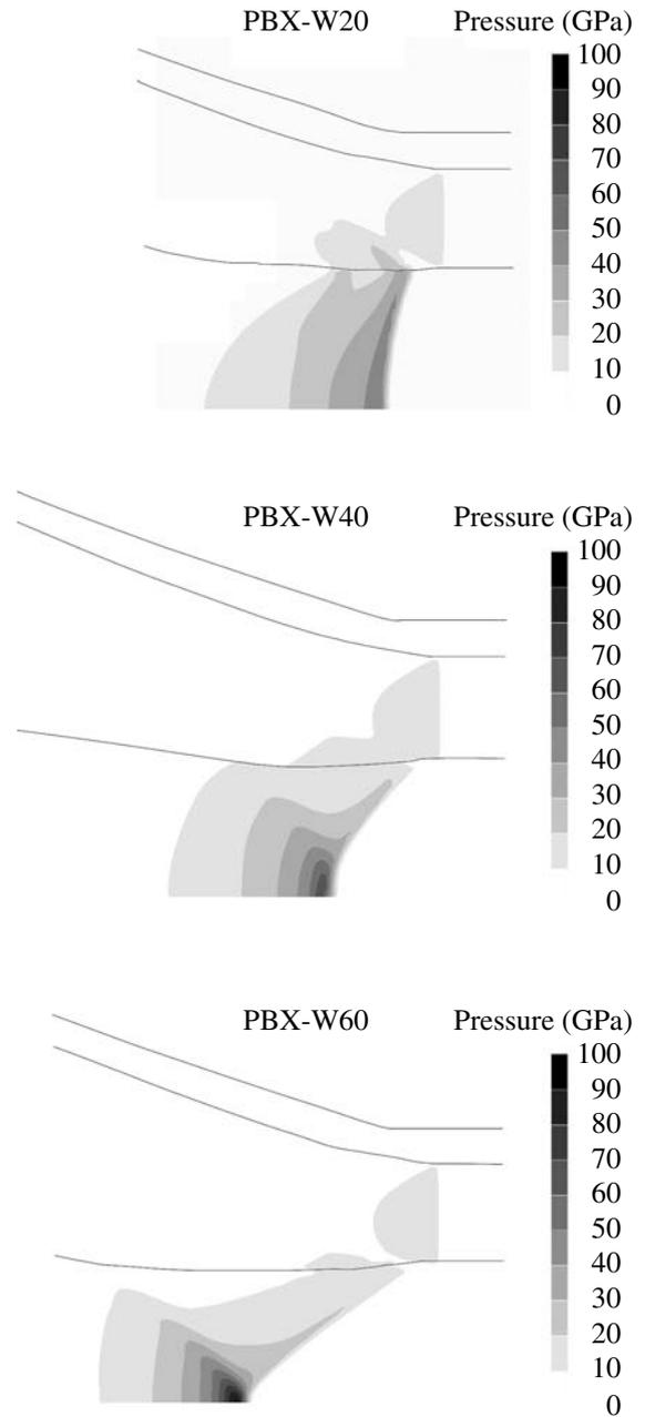
Fig. 10 Calculated pressure contours of the overdriven detonation.
