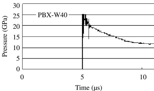
Fig. 3 Pressure profile by PVDF gauge.
