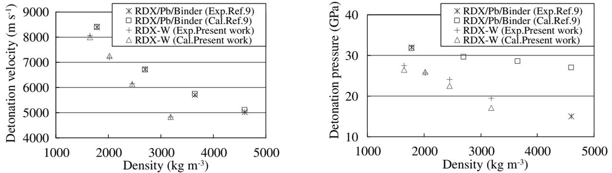
Fig. 5 Detonation properties of metal loaded explosives.
