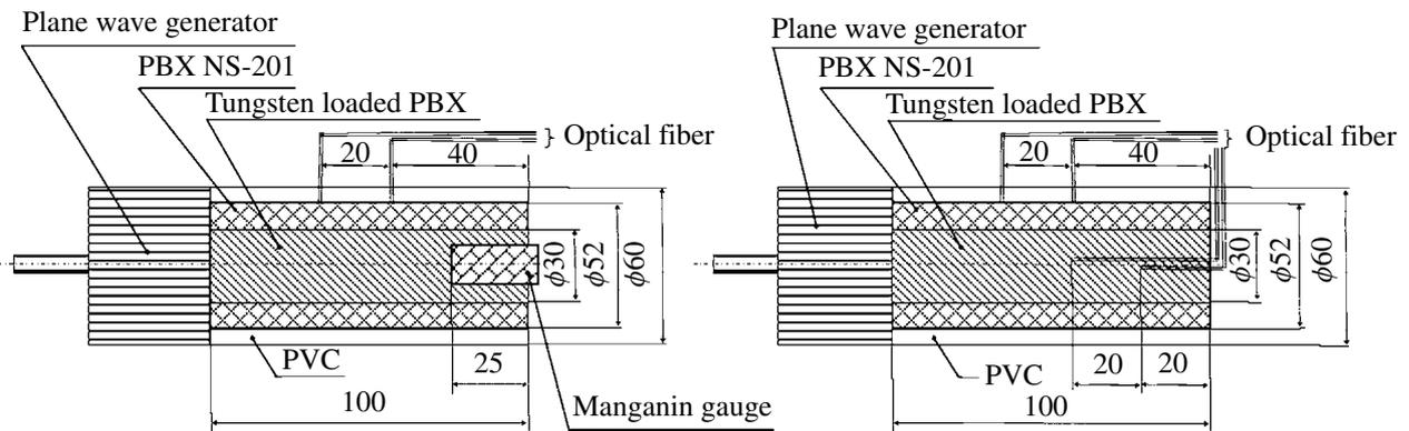
Fig. 6 Experimental devices to measure detonation velocity (right) and detonation pressure (left).
