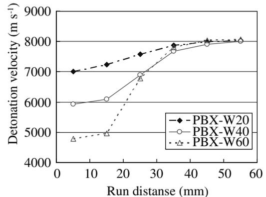
Fig. 8 Variation of the overdriven detonation velocity with run distance.
