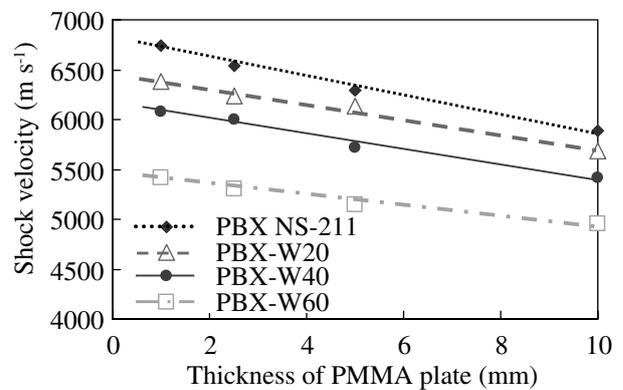
Fig. 2 Shock velocity in PMMA plate.
