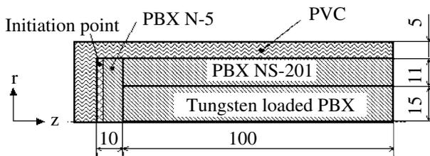
Fig. 7 Numerical simulation model.
