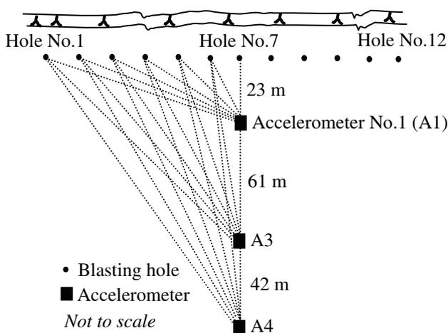
Fig. 4 The area of influence for each detonated hole.
