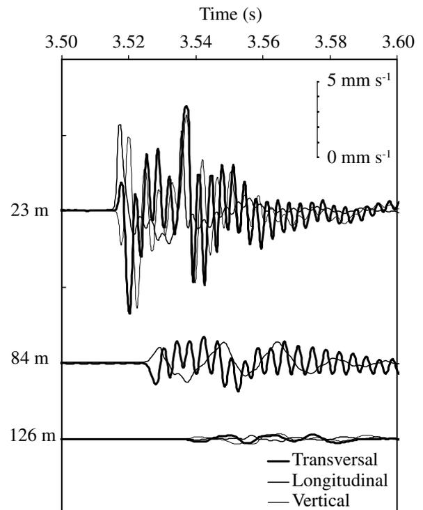
Fig. 5 A typical blast vibration waveform (zoom in).
