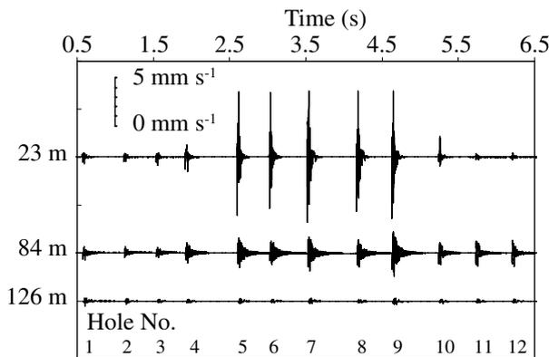
Fig. 3 A typical blast vibration waveform. (zoom out transverse motion)
