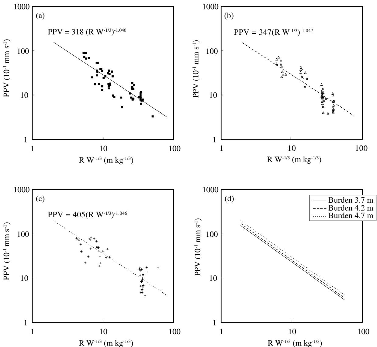
Fig. 7 PPV versus monitoring distance: (a) Burden 3.7 m; (b) Burden 4.2 m; (c) Burden 4.7 m; (d) All.
