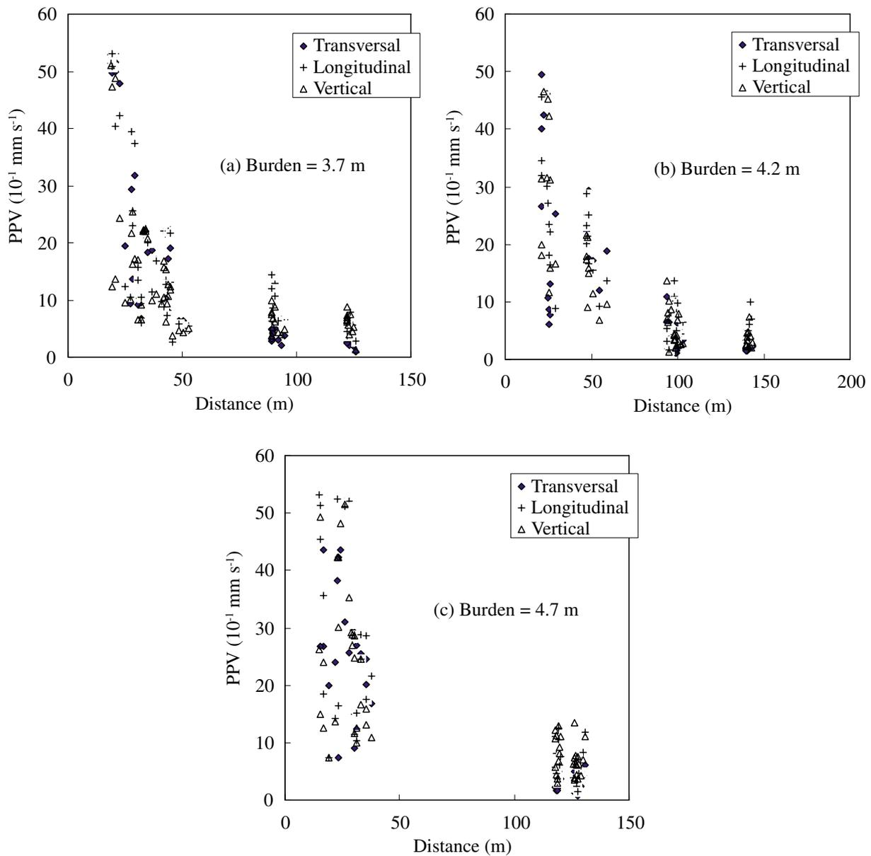
Fig. 6 PPV versus monitoring distance: (a) Burden 3.7 m; (b) Burden 4.2 m; (c) Burden 4.7 m.
