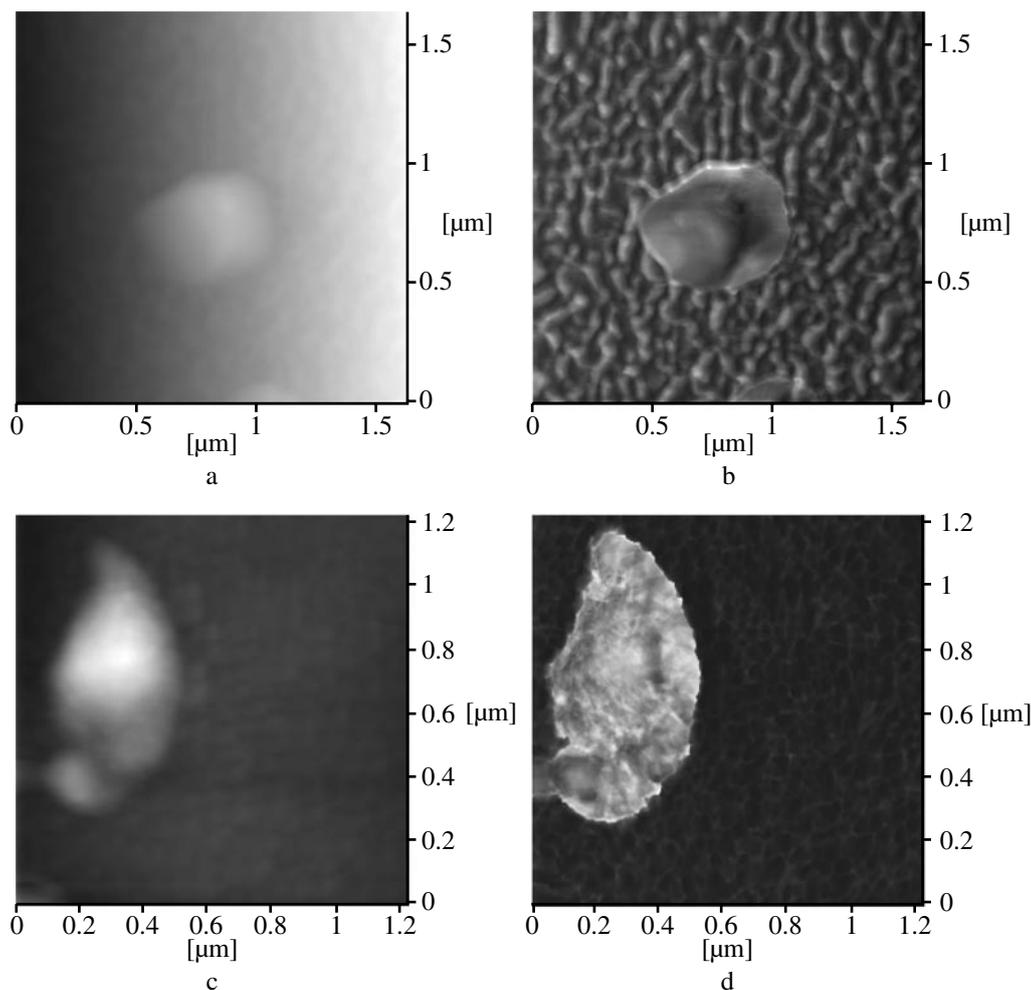
Fig. 2 AFM images. a: topography of ultrafine HMX, b: phase imaging of ultrafine HMX, c: topography of composite particle, d: phase imaging of composite particle.
