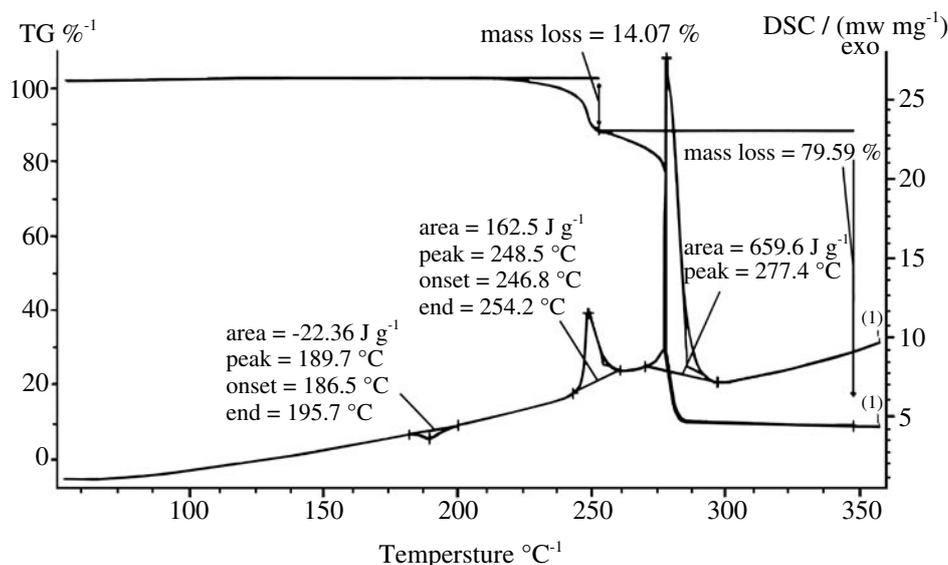
Fig. 4 TG-DSC curves for HMX/NTO composite particles. (Heat rate: 10 °C min<sup>-1</sup>. Atmosphere : argon at flow rate of 2 ml min<sup>-1</sup>. The sample amount: 1.4 mg)
