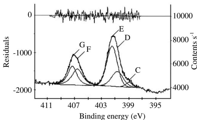
Fig. 3 N1s XPS spectrum for HMX/NTO core/shell composite particles.
