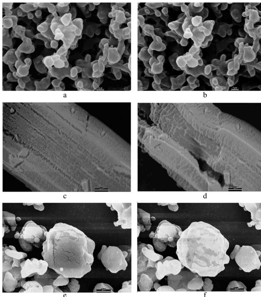
Fig. 1 SEM photographs of ultrafine HMX, NTO & HMX/NTO core/shell composite particles before and after exposure. (a: ultrafine HMX; b: ultrafine HMX after exposure; c: NTO particle; d: NTO particle after exposure; e: HMX/NTO core/shell composite particles ; f: HMX/NTO core-shell composite particles after exposure.)
