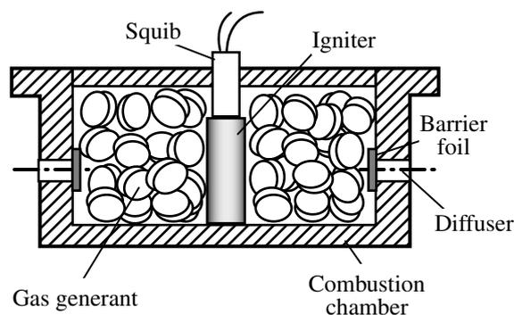
Fig. 4 Schematic diagram of combustion chamber.
