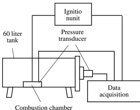
Fig. 5 Experimental setup for 60 liter tank test.
