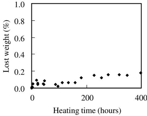
Fig. 8 Lost weight of pure GAT heated at 383 K.
