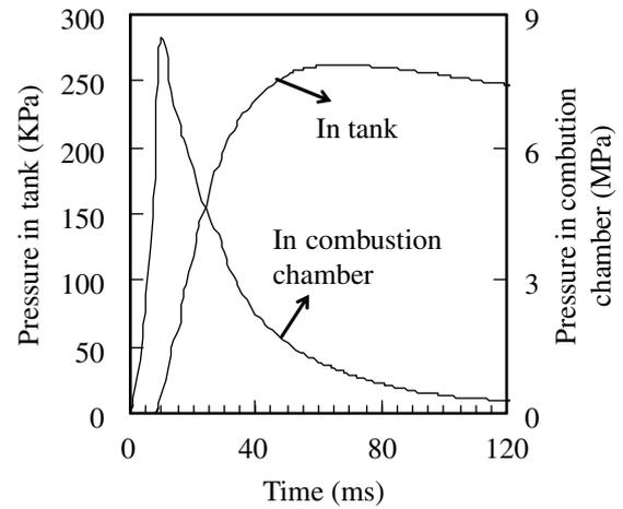
Fig. 9 Typical pressure profiles in combustion chamber and in 60 liter tank for GAT / Sr (NO<sub>3</sub>)<sub>2</sub>.
