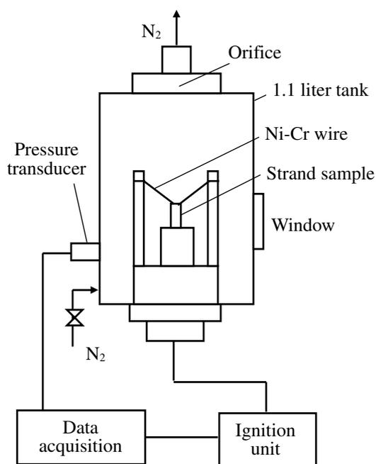
Fig. 2 Experimental setup for chimney-type strand burner.
