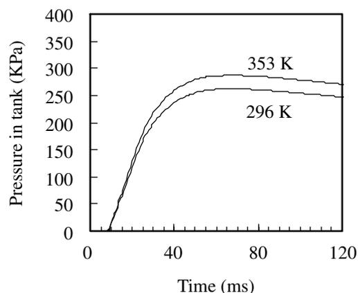
Fig. 10 Typical pressure profiles in 60 liter tank for GAT / Sr (NO<sub>3</sub>)<sub>2</sub> at 353 K and 296 K, respectively.
