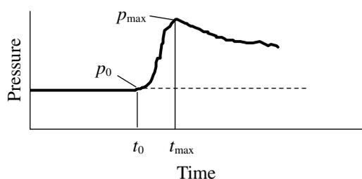
Fig. 3 Typical pressure profile in chimney-type strand burner. (burning time =  $t_{\max} - t_0$ )
