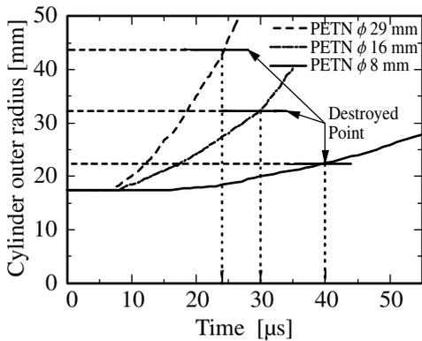
Fig. 6 Experimental wall radii for smooth cylinders.
