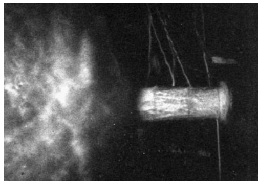
Fig. 4 High-speed photograph of detonation behaviour of ANFO using a glass tube. (Inner diameter: 40 mm)
