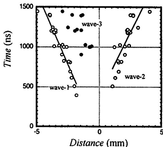
Fig. 3 The x-t diagram of the three wave fronts seen as in Fig. 2. Explosive thickness in all the data is about 0.5 mm.
