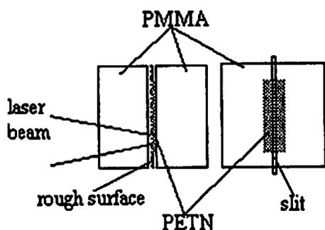
Fig. 4 Experimental setup for the streak shadowgraphy to observe the wave propagation along the thin explosive layer.
