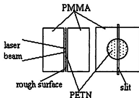
Fig. 1 Experimental setup for laser shadowgraphy of detonation induced stress wave in PMMA. Two thick PMMA plates of both sides are used to observe the induced high pressure stress wave in PMMA by explosion as well as to confine the explosive layer
