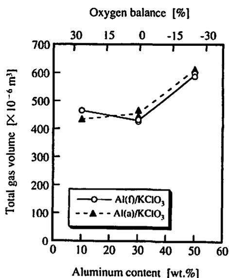
Fig. 3 Total gas volume obtained from the balloon test of Al/KClO<sub>3</sub> mixtures as a function of aluminum content
