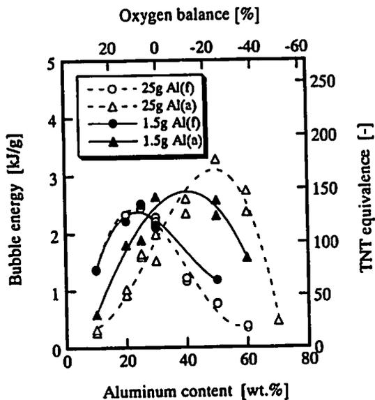
Fig. 7 Bubble energies of Al/KClO<sub>3</sub> mixtures as a function of aluminum content
