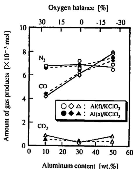
Fig. 4 Influence of aluminum content of the amount of gas products (N<sub>2</sub>, CO, CO<sub>2</sub>) obtained from the balloon test of Al/KClO<sub>3</sub> mixtures
