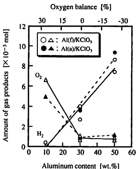
Fig. 5 Influence of aluminum content on the amount of gas products ( $H_2, O_2$ ) obtained from the balloon test of  $Al/KClO_3$  mixtures
