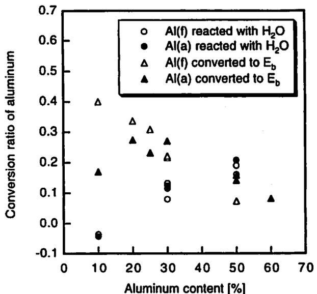
Fig. 8 Conversion ratio of aluminum to the reaction with water and to the bubble energy as a function of aluminum content of Al/KClO<sub>3</sub>
