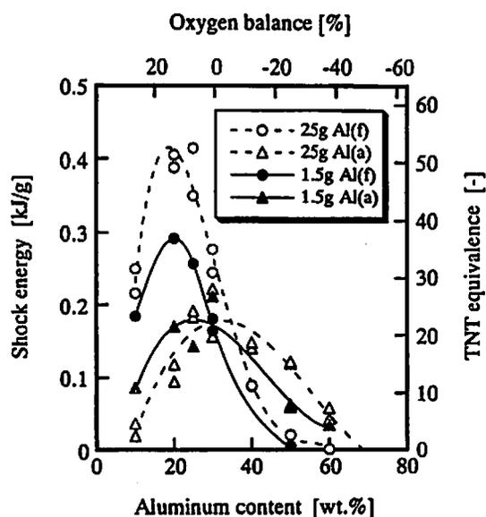
Fig. 6 Shock energies of  $Al/KClO_3$  mixtures as a function of aluminum content
