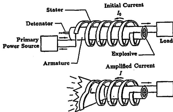
Fig. 1 Operation principle of the explosive-driven magnetic flux compression generator ; before (upper) and during operation (lower)
