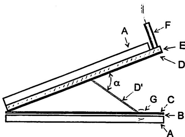
Fig. 4 A schematic view of a device for the flight angle measurement. A:Acrylic acid resin plate, B:argon gap, C:steel shim, D:driver plate, E:explosive sheet, F:detonator. The broken line(D') illustrates how the driver plate(D) would be deformed some time after the initiation. The angle  $\alpha$  is the flight angle and argon gas in the gap(B) around the area 'G' emits a flush light.
