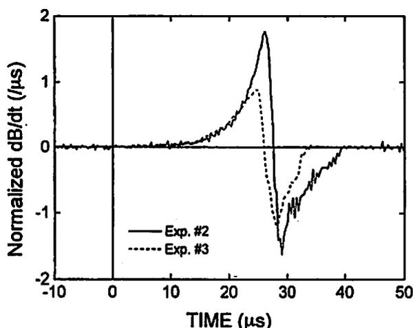
Fig. 8 Time derivatives of the magnetic fields normalized by the initial fields vs. time in experiments #2 and #3. In both curves, compression start time is set at zero.
