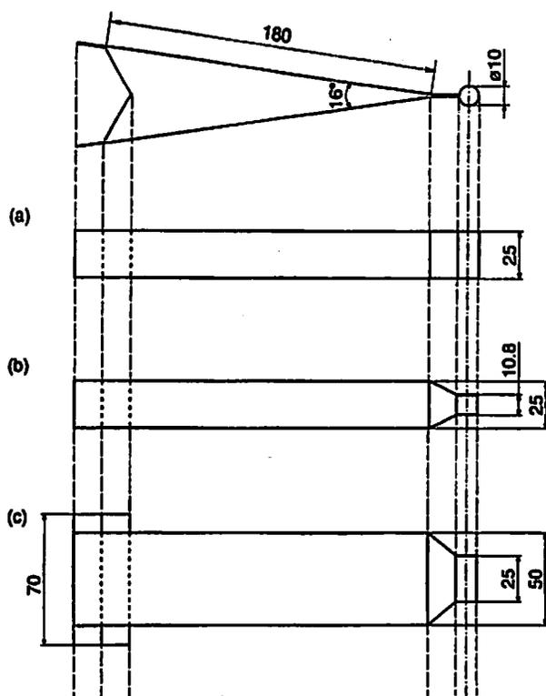
Fig. 3 Shape of the bellow coils employed in this work. The thickness of the copper plate was always 0.5mm.
