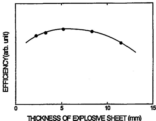
Fig. 5(b) The explosive sheet thickness dependence of the efficiency of the driver plate acceleration by the explosive sheet. A solid line is only aids to the eye.
