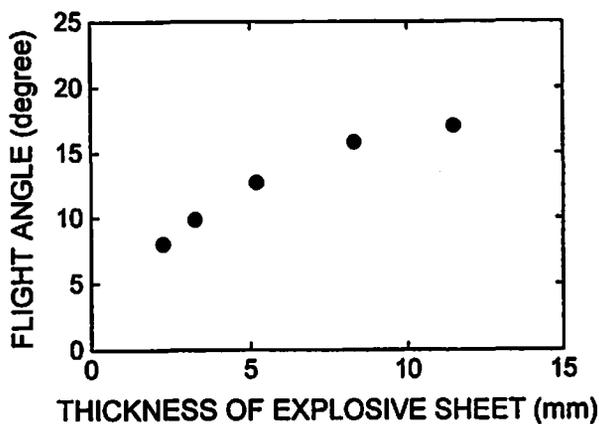
Fig. 5(a) The flight angle of a driver plate vs. the square root of the explosive sheets thickness ( $t$ ). The driver plate was a 0.5mm thick copper plate. The explosive sheets were made of PETN bonded by silicon rubber in the weight ratio of 7 : 3.
