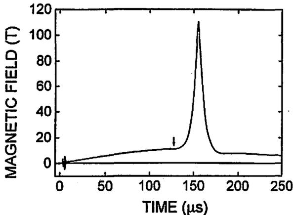
Fig. 6 Time variation of a magnetic field measured in the center of the load coil in experiment # 5. The flux compression started at  $127.9\mu\text{s}$  (indicated by the arrow) when the initial field was  $10.9\text{T}$  and the field increased up to  $110.7\text{T}$  after  $27.3\mu\text{s}$ .
