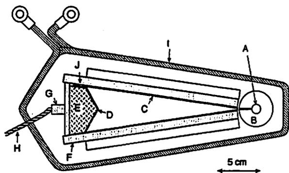
Fig. 2 A schematic view of the bellows-type flux compression device. A:load coil, B:collar, C:driver plate, D:base plate, E:base block, F:explosive sheet, G:booster, H:detonation cord, I:external coil, J:gap.
