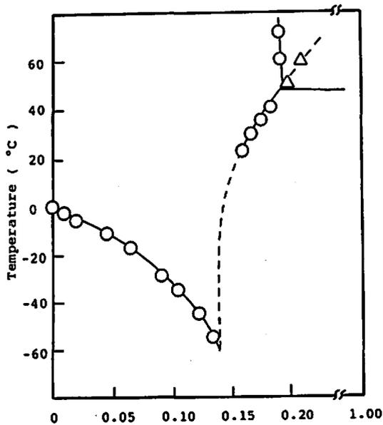
Fig. 1 Solubility curve of  $\text{LiClO}_2$  in water
