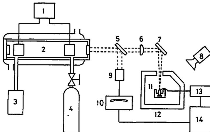
Fig. 2 Schematic diagram of CO<sub>2</sub> laser ignition apparatus.
