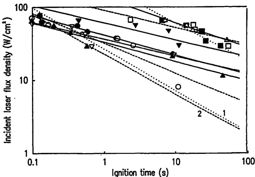
Fig. 3 Relation between incident laser flux density and ignition time
