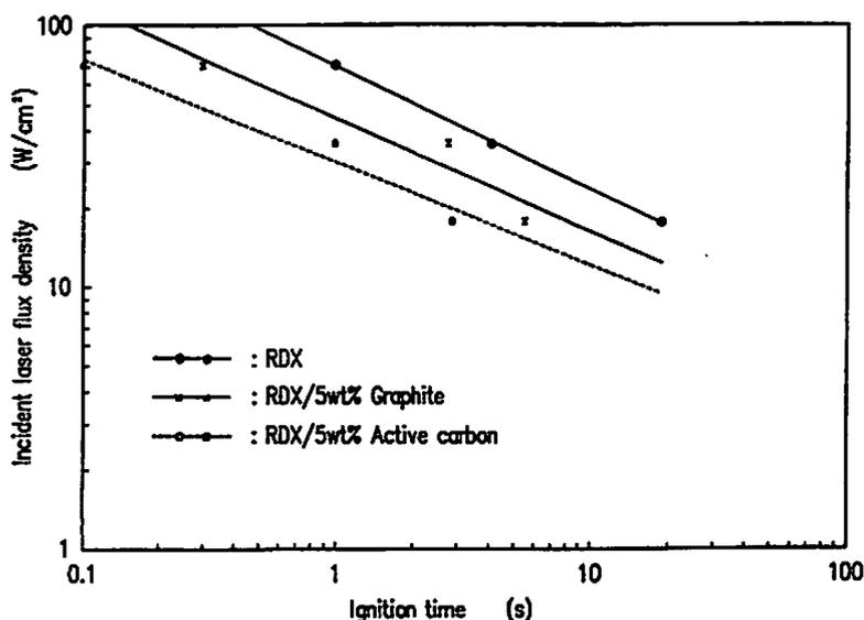
Fig. 4 Effect of additives on ignition of RDX
