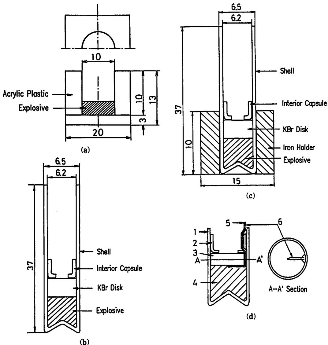
Fig. 1 Cross-sectional view of the containers
