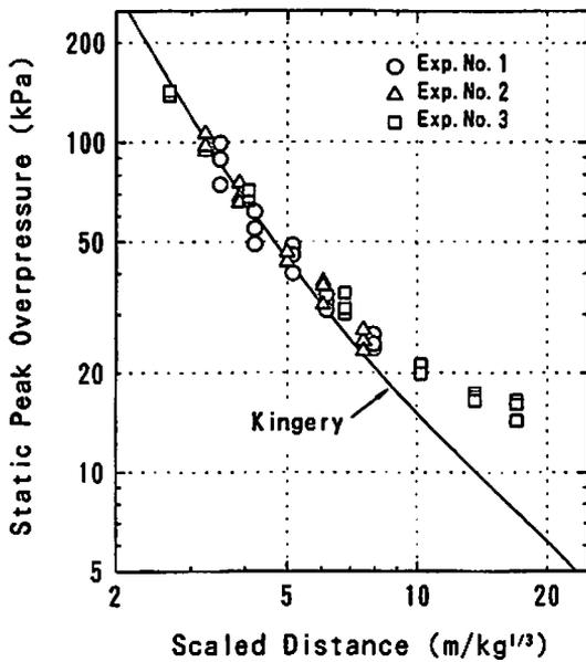
Fig. 2 Static peak overpressure of TNT blast waves measured by blastmeter (Type C) calibrated with the original calibration table
