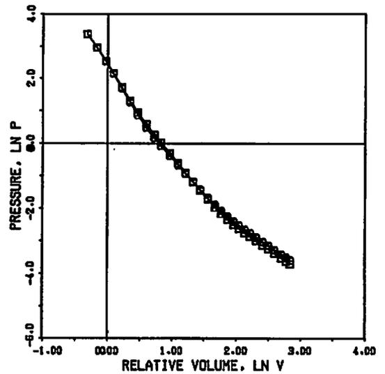
Fig. 7 Comparison of p-V curve for comp-B obtained with our method (○) and LLNL (□)
