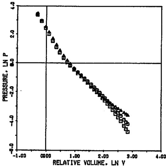
Fig. 6 Comparison of p-V data for comp-B calculated by our method including metal strength (○) and not including the metal strength (□) and LLNL (△)
