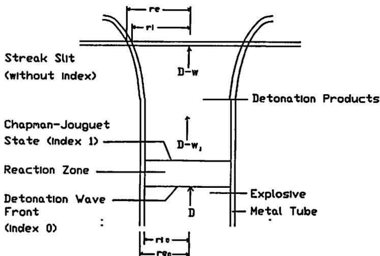
Fig. 1 Flow conditions of the detonation products in expanded metal cylinders
