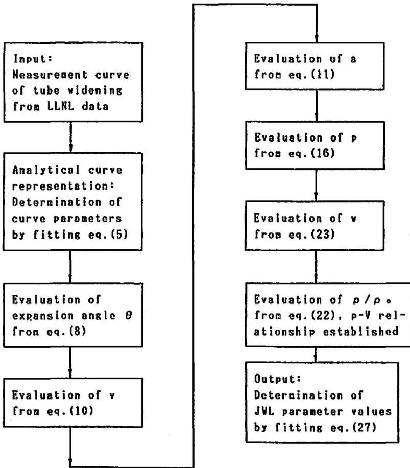
Fig. 4 Flow chart of our calculation procedure
