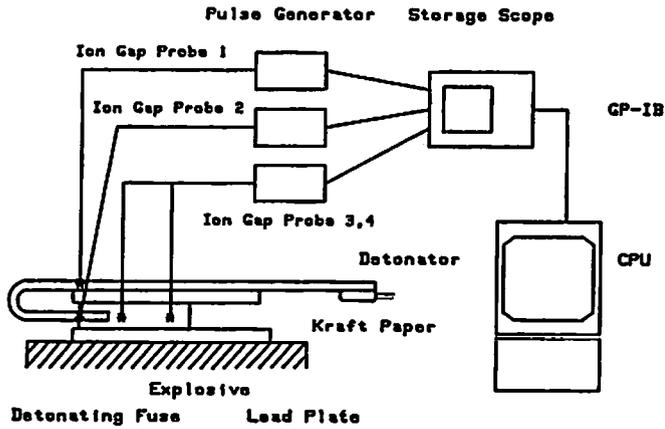
Fig. 1 Measuring system for experiment
