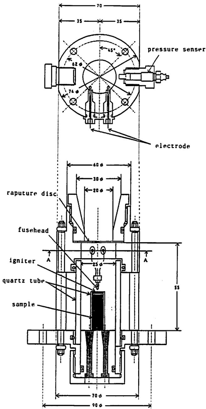
Fig. 1 Cross-section of visible type Time-Pressure test apparatus.
