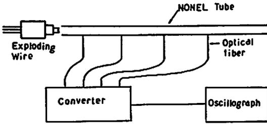
Fig. 1 Schematics of experimental configuration
