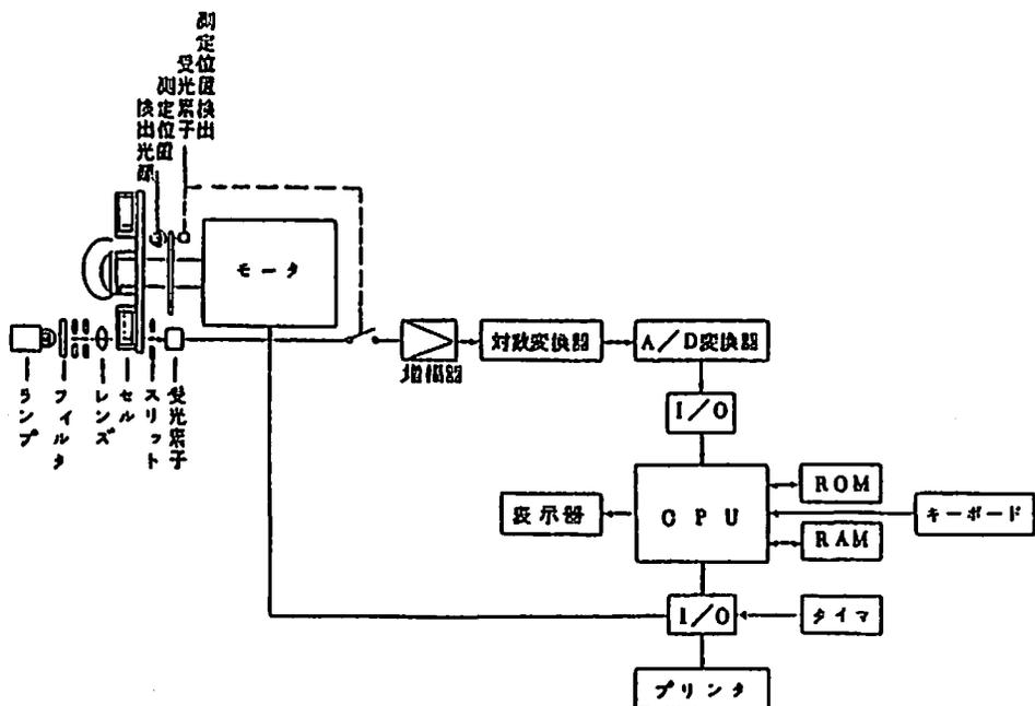
Fig. 1 Schematic diagram of centrifugal particle size analyzer combined with a microcomputer
