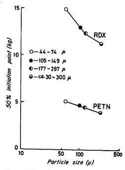
Fig. 6 Effect of particle size on the friction sensitivity of PETN and RDX
