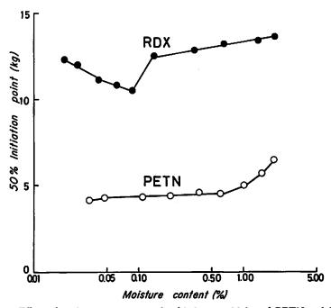
Fig. 5 Effect of moisture content on the friction sensitivity of PETN and RDX
