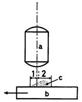
Fig. 2 Position of the test sample on the porcelain plate
