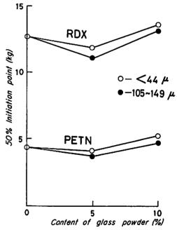
Fig. 7 Effect of glass powder added as grit on the friction sensitivity of PETN and RDX
