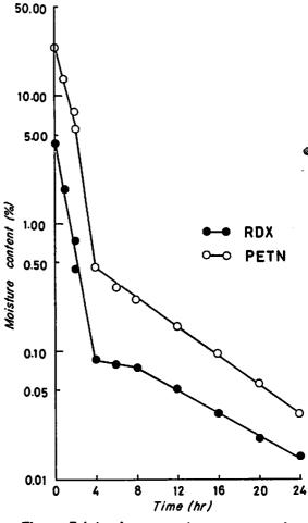
Fig. 3 Relation between moisture content and drying time
