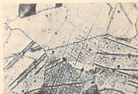
Photo. 1. Microstructure showing two or three directions of Neumann bands in ferrite grains very near the outer free surface. ( \times 280 ).
