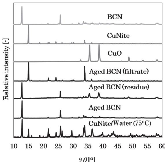
Figure 2 XRD pattern of aged BCN samples (Aging span: 2 [h]).
