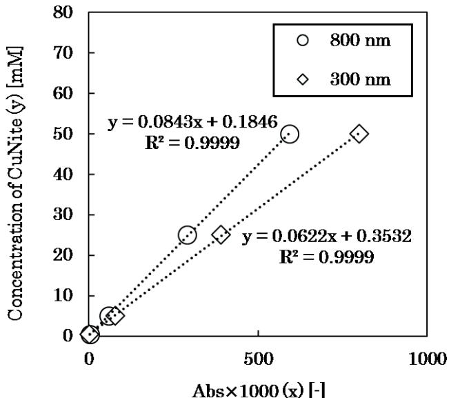
Figure 5 Calibration line of CuNite solution.
