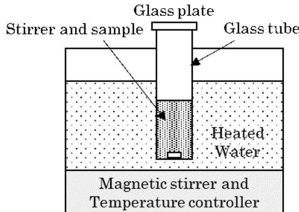
Figure 1 Schematic of accelerated aging test.
