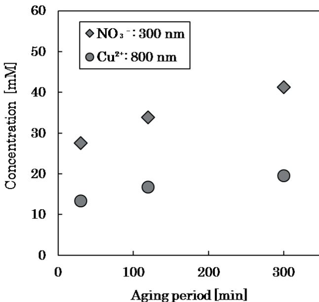
Figure 6 Quantitative analysis of Cu<sup>2+</sup> and NO<sub>3</sub><sup>-</sup> in aged BCN (filtrate).
