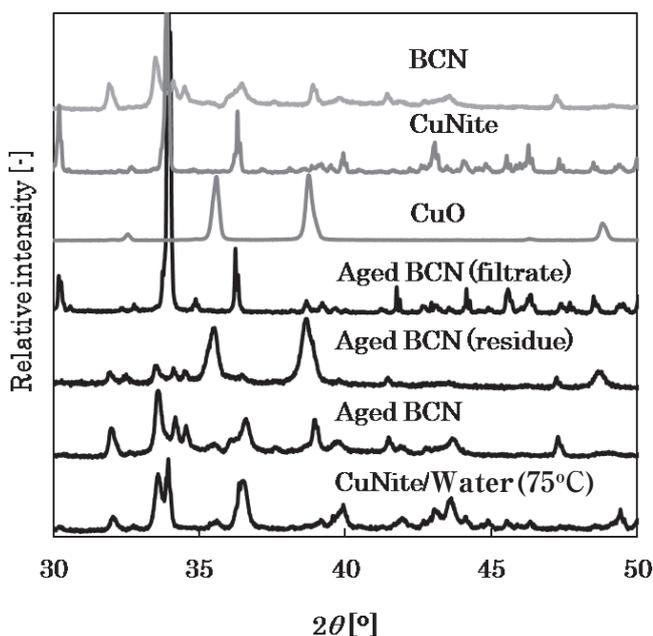
Figure 3 XRD pattern of aged BCN samples (Aging span: 2 [h]) [Enlarged around CuO peaks].
