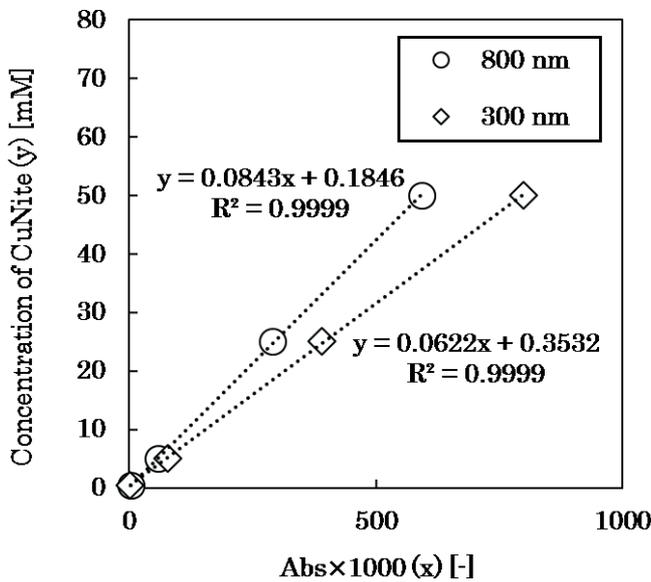
Figure 5 Calibration line of CuNite solution.
