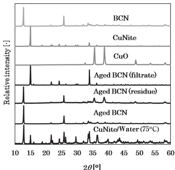
Figure 2 XRD pattern of aged BCN samples (Aging span: 2 [h]).
