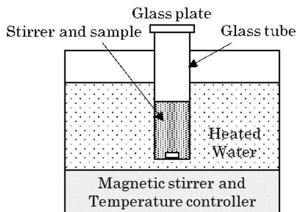
Figure 1 Schematic of accelerated aging test.
