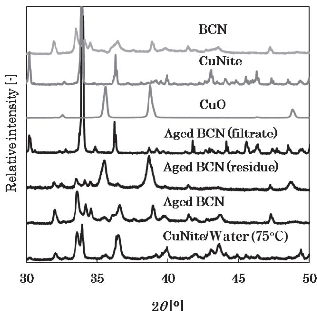
Figure 3 XRD pattern of aged BCN samples (Aging span: 2 [h])
