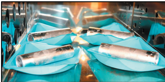
Figure 3 Al cylinders were coated with gallium and were held at an elevated temperature in an oven (4 cylinders shown).
