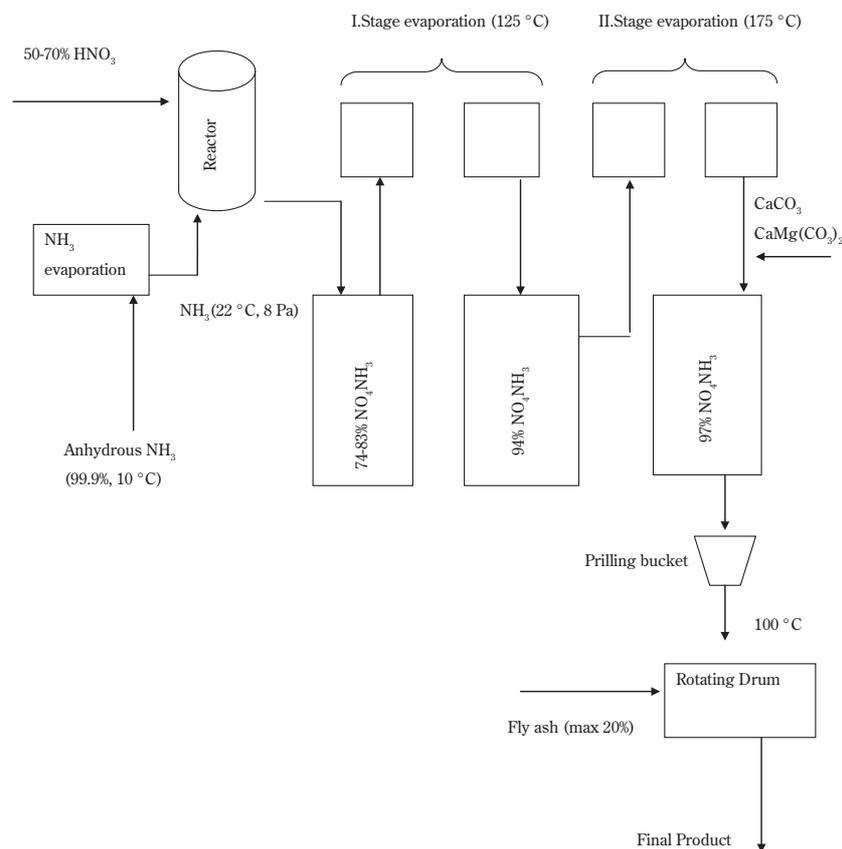
Figure 1 Fertilizer manufacturing process involving two evaporation stages.
