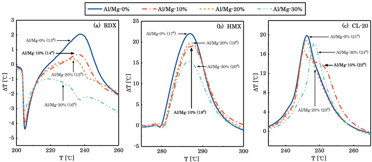
Figure 2 DTA curves of three kinds of explosives with different mass percentages of Al-Mg alloy powder.
