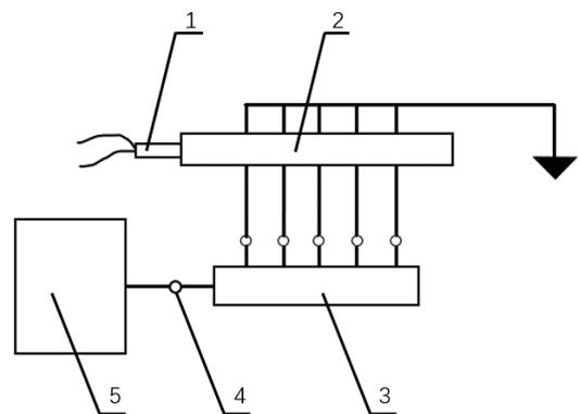
Figure 4 Connection between specimen and instrument (1-Detonator; 2-Specimen; 3-Pulse forming network; 4-Wire; 5-Timer).
