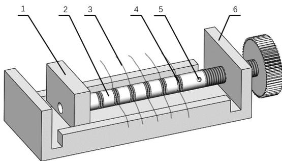
Figure 3 Installation of explosive columns in the wooden trough (1-Wooden trough; 2-Explosive column; 3-Probe; 4-Sponge cushion; 5-Timber column; 6-Top pressure device).
