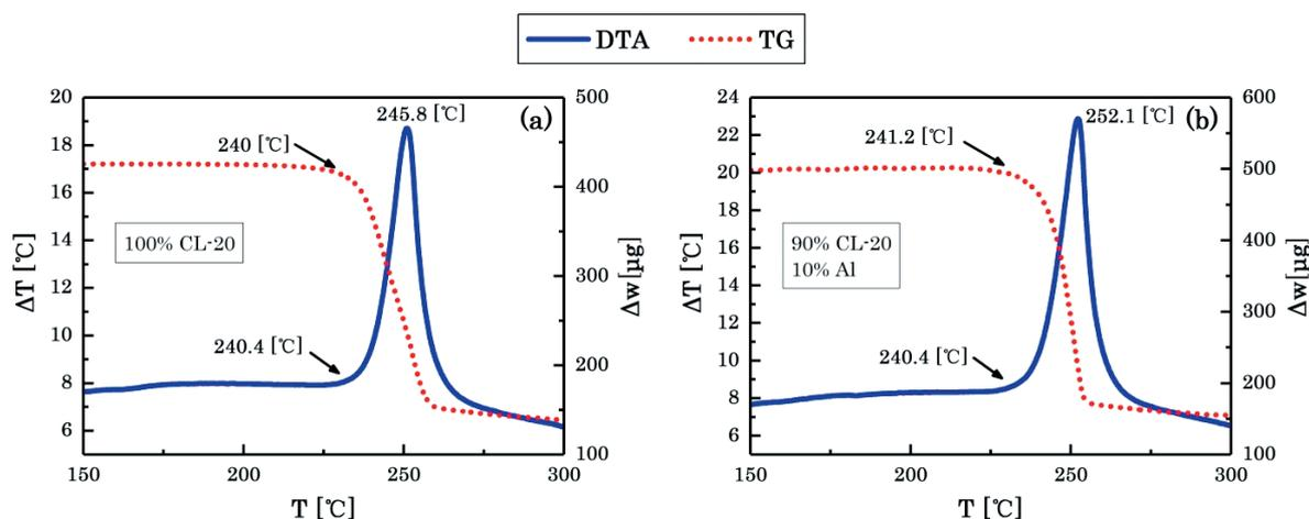
**Figure 6** TG-DTA curves of CL-20 before and after addition of aluminum powder (a: Pure CL-20; b: CL-20 90 wt% and Al 10 wt%).
