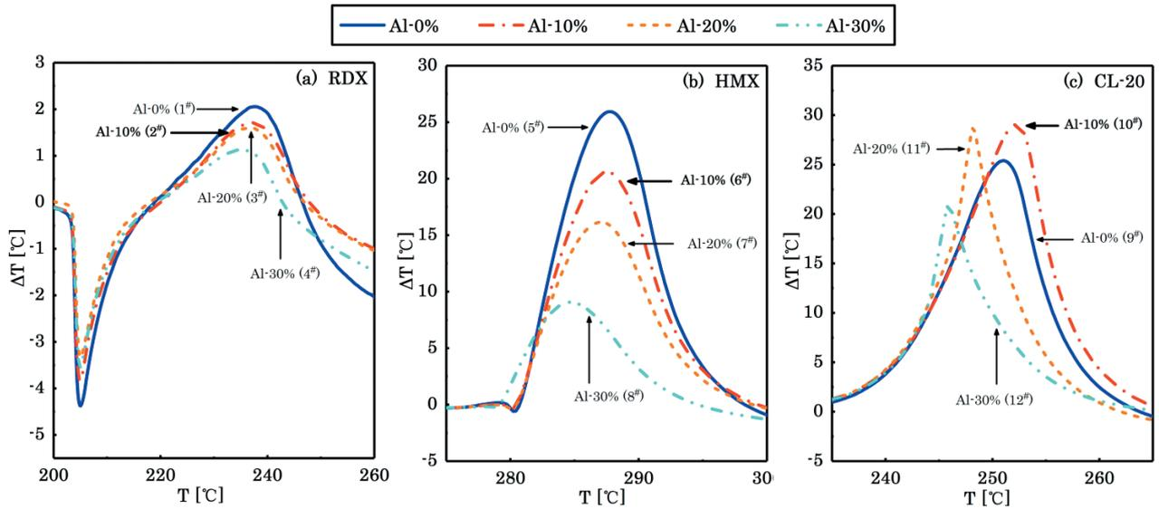
Figure 1 DTA curves of three kinds of explosives with different mass percentages of Al powder.
