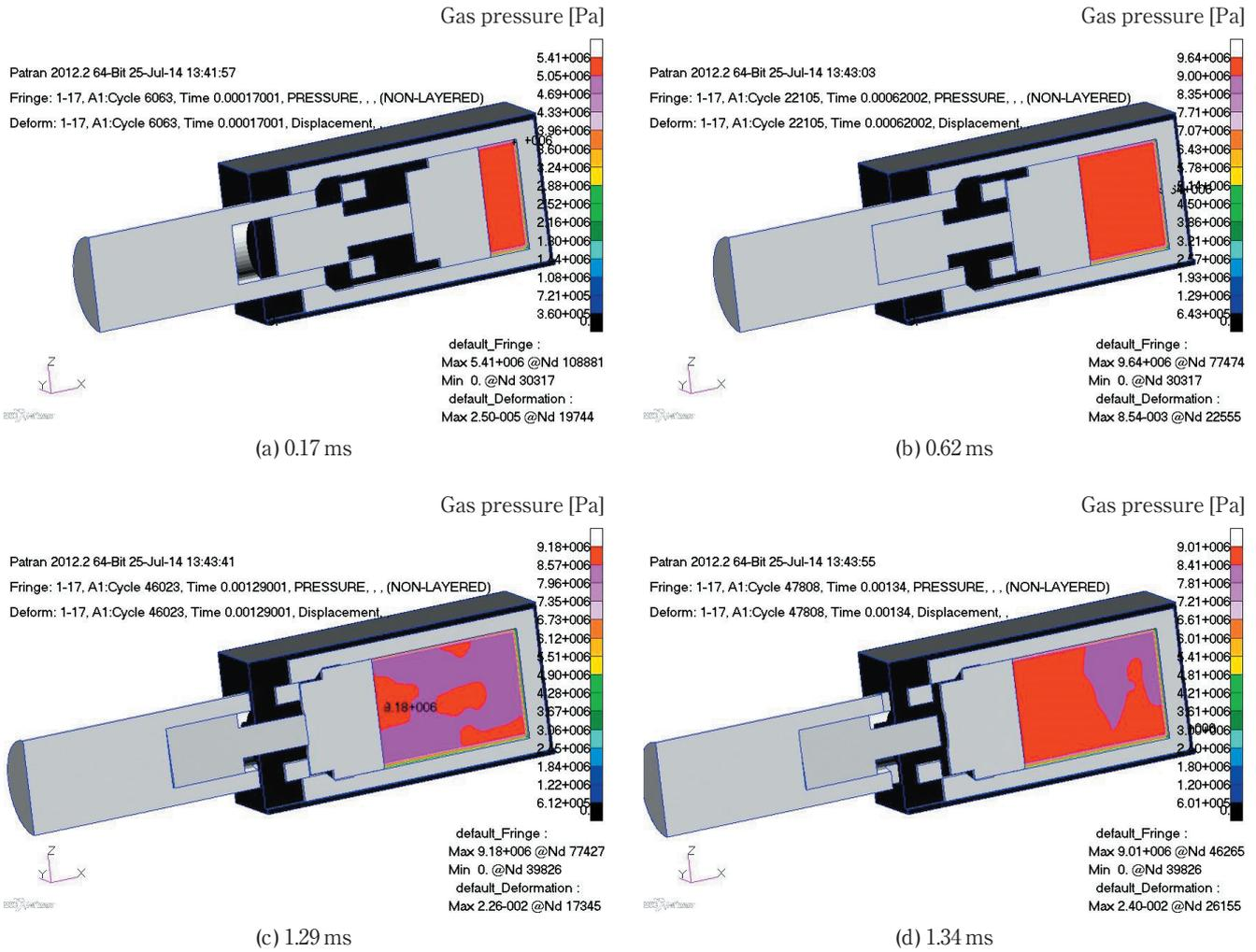
Figure 8 The movement process of catapult at different moments.
