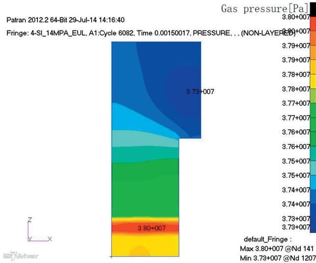
Figure 6 The calculation pressure contour.
