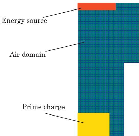
Figure 3 Numerical model of closed vessel.
