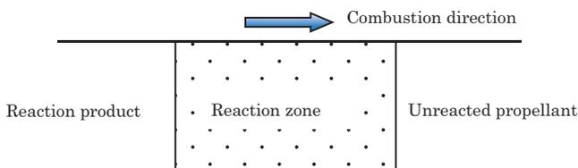
Figure 1 Scheme of classic propellant burn.
