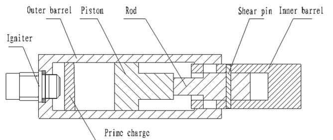
Figure 4 Geometry of the catapult.
