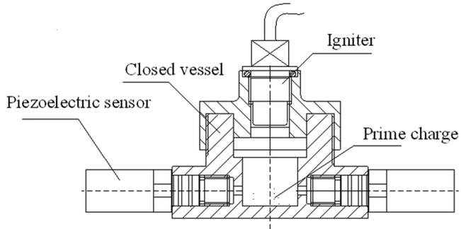
Figure 2 Geometry of closed vessel test.
