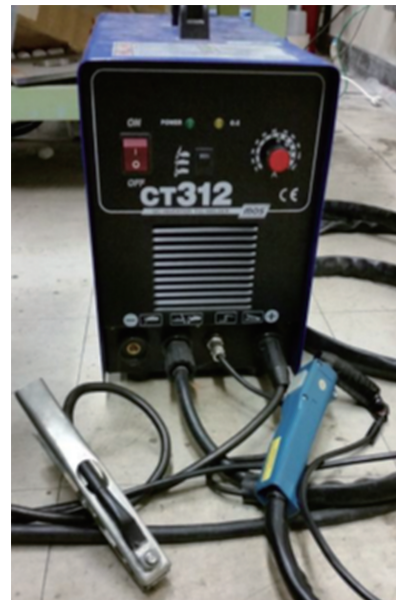
Figure 3 Power unit of plasma torch.
