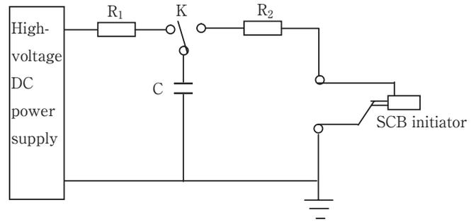
Figure 5 Schematic diagram of ESD experiment.
