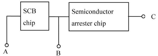
Figure 2 Pin-to-case ESD protection for SCB initiator.
