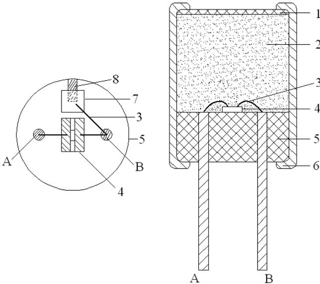
Figure 4 (a) Sketch diagram of SCB packaged semiconductor arrester chip.
