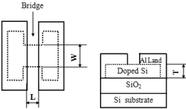
Figure 3 Simplified sketch of SCB chip.
