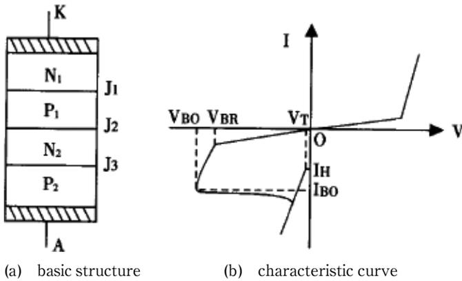
Figure 1 Diagram of the basic structure and characteristic curve of semiconductor arrester chip.
