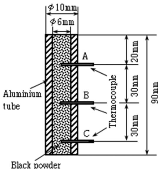
Figure 1 Setup of temperature measurement.
