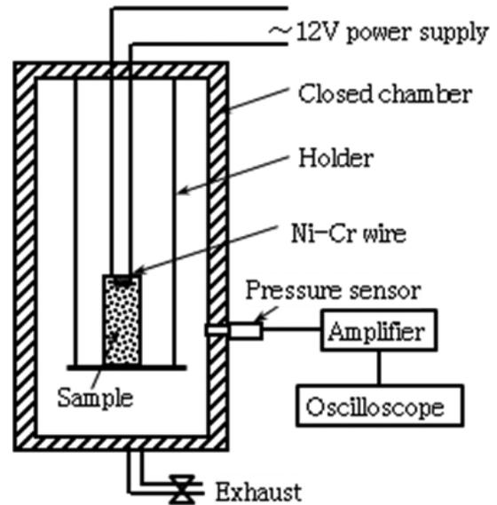
Figure 2 Setup of closed tank test.
