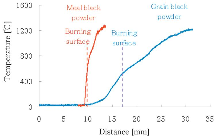
Figure 4 Temperature profile of grain and meal black powder.
