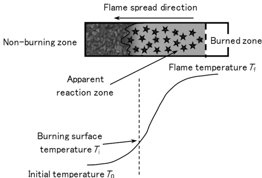
Figure 6 A schematic diagram for burning grain black powder.
