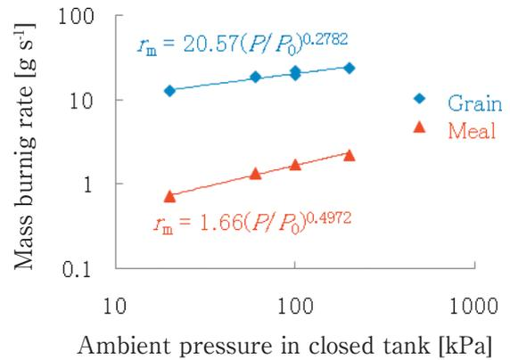
**Figure 7** Relationship between mass burning rate and ambient pressure.
