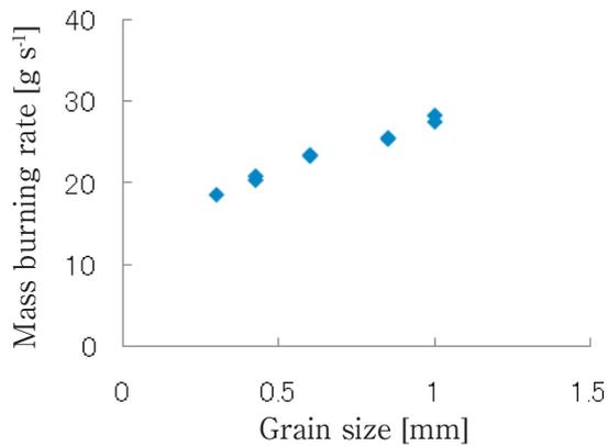
**Figure 8** Mass burning rates of black powder with various grain sizes.
