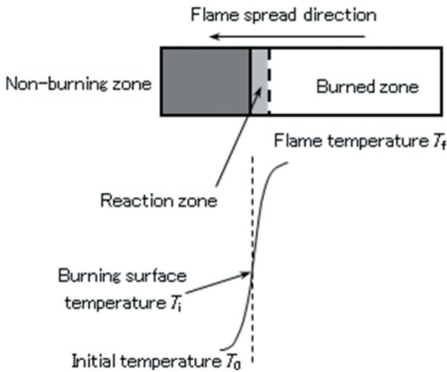
Figure 5 A schematic diagram for the burning meal black powder.
