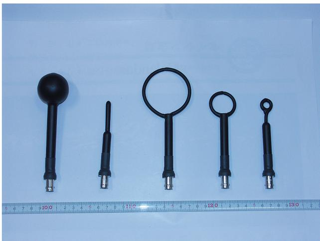
Fig. 2 Sensors to observe igniting sparks.
