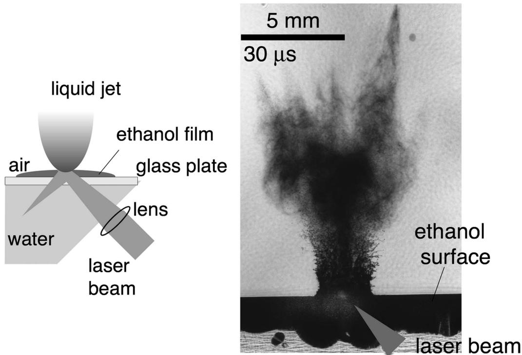
**Fig. 2** Schematic of experimental assembly and laser shadowgraph reproduction of the laser ablation of ethanol surface. Delay time of the record is shown in the photograph. Laser energy is 300 mJ and laser fluence is calculated to be  $20 \text{ J cm}^{-2}$ .
