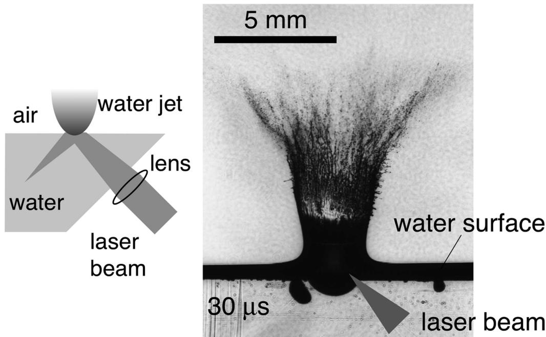
**Fig. 1** Schematic of experimental assembly and laser shadowgraph reproduction of the laser ablation of water surface. Laser beam is focused from bottom right to the air interface and reflected to the breakdown region. Delay time of the record is shown in the photograph. Laser energy is 300 mJ and laser fluence is calculated to be  $20 \text{ J cm}^{-2}$ .
