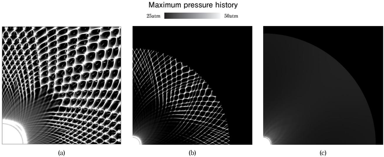
Fig. 2 Maximum pressure histories in the case of  $r_s=700\mu\text{m}$ . The grid sizes are (a)  $2.5\mu\text{m}$ , (b)  $5.0\mu\text{m}$ , and (c)  $10.0\mu\text{m}$  for each case. The range of pressure is between 25 and 50atm.
