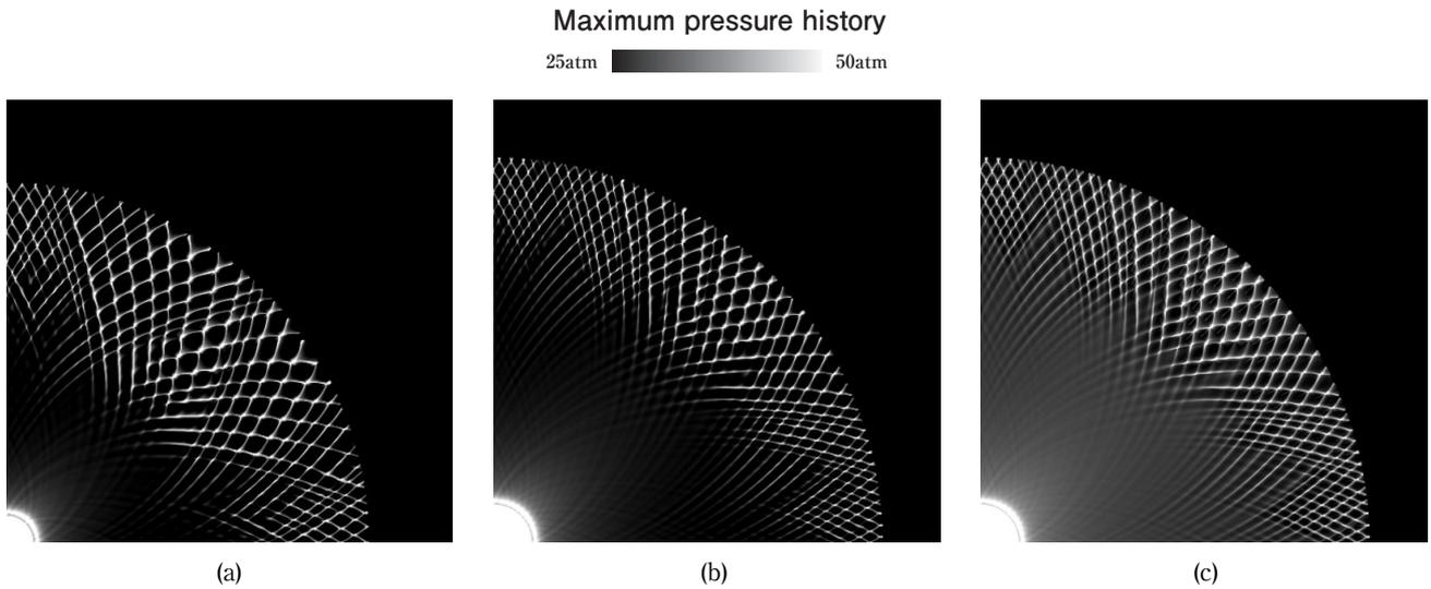
Fig. 3 Maximum pressure histories for  $\Delta x=5.0\mu\text{m}$  in the case of (a)  $r_s=500\mu\text{m}$ , (b)  $r_s=700\mu\text{m}$ , and (c)  $r_s=900\mu\text{m}$ . The range of pressure is between 25 and 50atm. The white lines denote the tracks of triple points.
