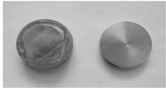
Fig. 5 A typical photo of damaged free surface of recovered momentum trap MT (left) and momentum side surface of recovered test specimen TP (right) for direct incidence type test (TP10 / MT15) of SUS304.
