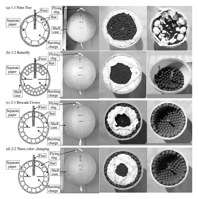
Fig. 1 Cross section and photograph of 240 mm color shell (*Warimono* (spherical) shell).
