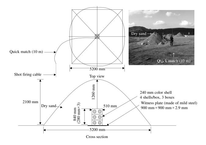
Fig. 2 Experimental setup for the gap test in sand.
