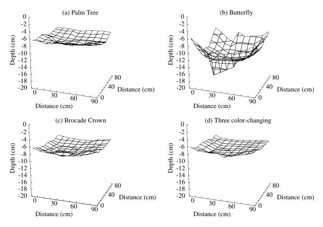
Fig. 4 Distortion situation on the witness plates.
