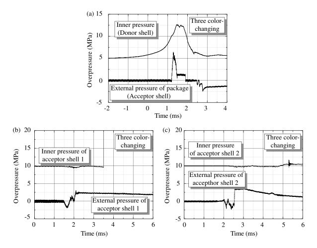
Fig. 6 Pressure change of the 240 mm color shell (Three color-changing).
