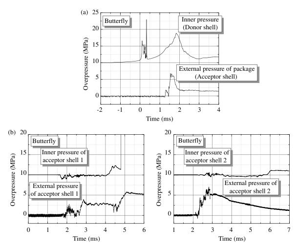
Fig. 5 Pressure change of the 240 mm color shell (Butterfly).
