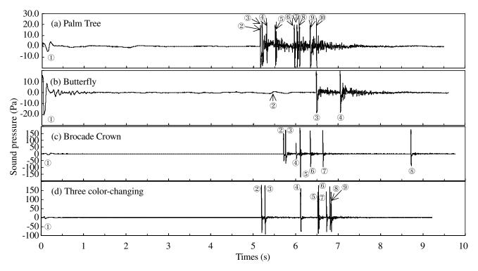
Fig. 7 Sound pressure waveforms of the explosion noise obtained by the gap tests in sand of the 240 mm color shells.
