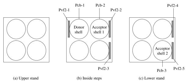
Fig. 3 Mounting position of the pressure sensors.
