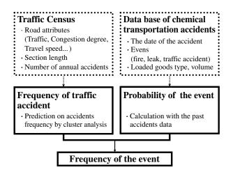
Fig. 1 Prediction scheme of the frequency of dangerous goods transportation.
