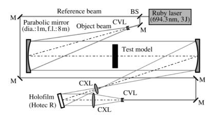
M: mirror, BS: beam splitter, CVL: concave lens, CXL: convex lens
