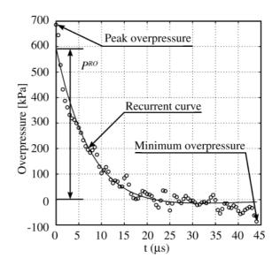
Fig. 5 Representative overpressure profile produced by Silver-azide explosion.
