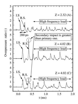
Fig. 9 Overpressure profile over the walls in R-I.
