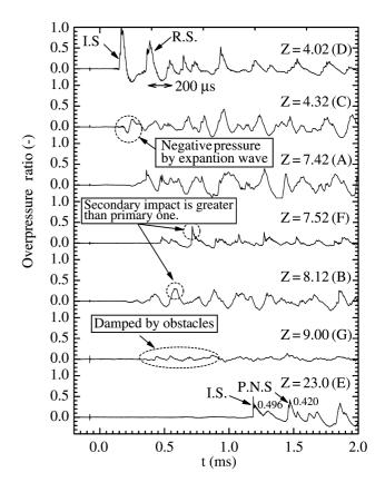
Fig. 10 Overpressure profile over the walls in the test model.
