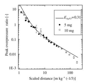
Fig. 6 Peak overpressure as a function of scaled distance for Silver-azide.
