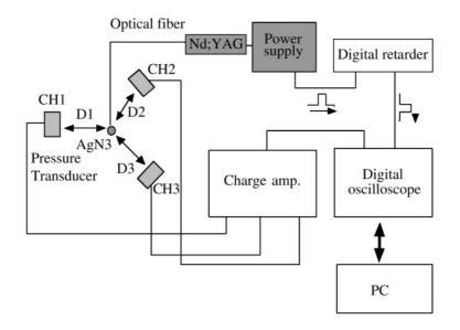
Fig. 2 Schematic of overpressure measurement system.
