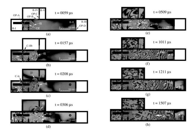
Fig. 8 Interferograms of shock waves propagation in the test model .
