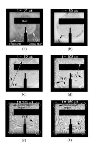
Fig. 7 Interferograms of shock waves propagation in R-I.
