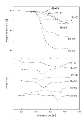
Fig. 3 TG-DTA results for lead picrates (upper column: TG, lower column: DTA).
