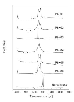
Fig. 2 DSC results for lead picrates.
