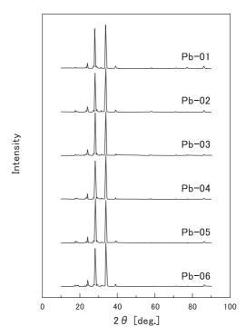
Fig. 4 X-ray fluorescence analysis results for lead picrates (spectrum crystal: LiF, wavelength range: 10–90°).
