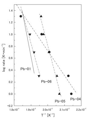
Fig.6 Ozawa's plots for decomposition start temperatures of lead picrates.
