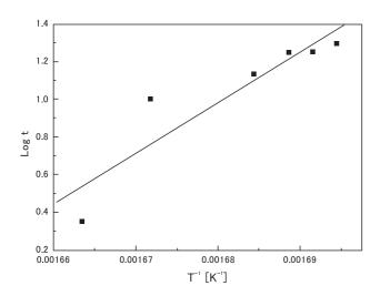
Fig. 7 Ignition temperature test results for Pb-04 (T: ignition temperature [K], t: time to ignite [s]).
