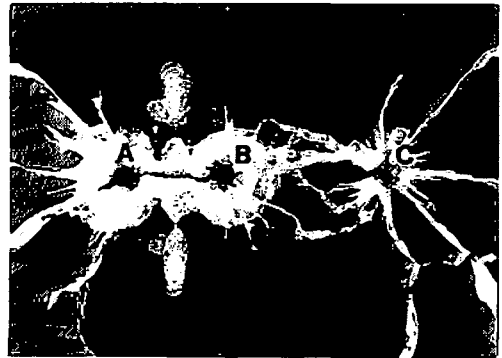
Fig. 7 Photograph of smooth blasting in the acrylic resin plate using precise blasting machine
