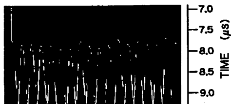
Fig. 6 Streak camera record of light emission from the argon gap at the bottom of detonators indicated in Fig. 3. Ten of twenty-four detonators were within the field of view of a camera.
