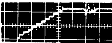
Fig. 2 An example of Oscillograms (TNT Slurry) (Sweep speed : 100 \mu sec/div.)
