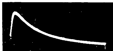
Photo. 2. Duration of explosion flame of a detonator (by Kato)
